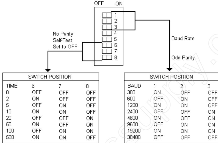
Dipswitch 2 sets the communication protocol and communication functions. Switch 1 and 2 select the protocol to be used. The following table shows the valid switch setting for the Operator Station Interface.
