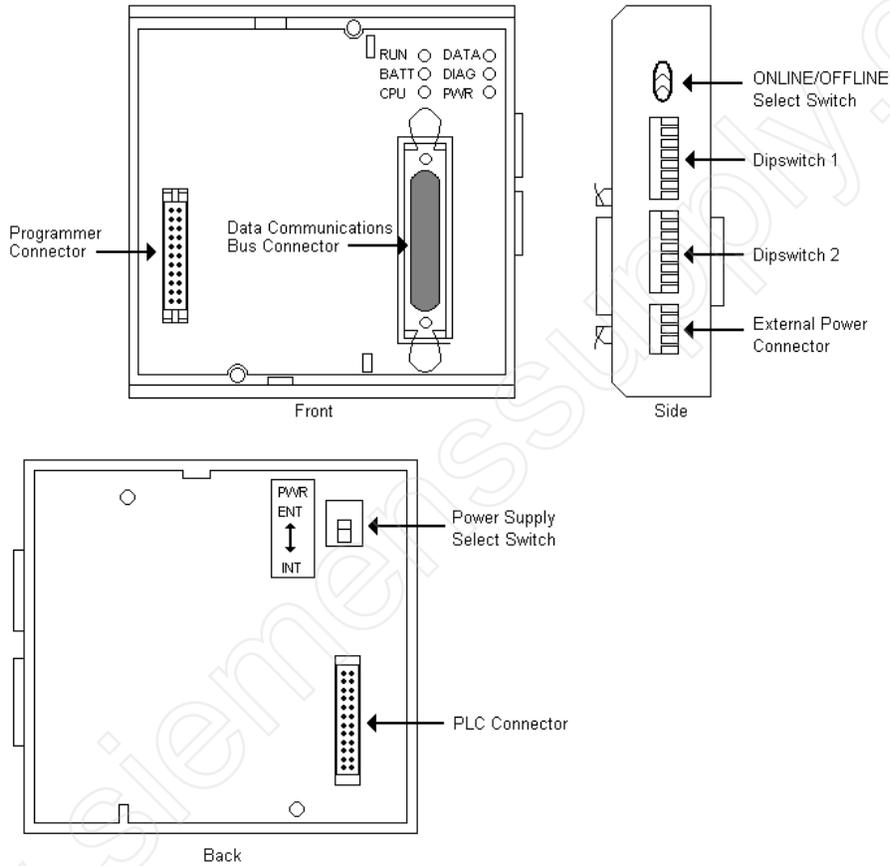
There are two dipswitches located on the DCU. Dipswitch 1 selects the baud rate and internal functions. Switches 1 and 2 of dipswitch 1 select the baud rate. Switches 3 through 8 select the internal functions of dipswitch 1. See the following tables for the recommended settings.
