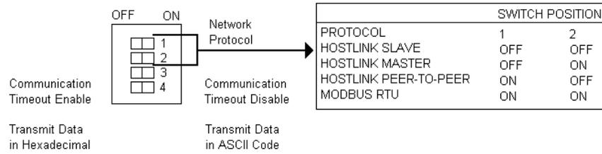
The following parameters are the default port characteristics of the DCM.
